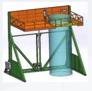
The [20-400] cells that compose the stack are stacked vertically, one piece at a time. In this crucial step, ensuring perfect alignment is key
